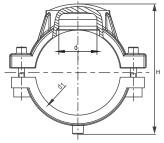
Repair and reinforcement saddle RSV SDR 11
