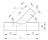
Unequal branch with reduced outlet 45°, SDR 17 (spigot fitting) ATSR 45
