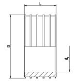
Shaft lining adapter for sewage inspection chambers L = 250 mm ASFL
