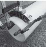
Maximum shear load per FIXBLOC: 40 kN
