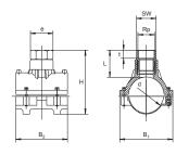
Valve tapping saddle with transition HD-PE/gunmetal VAM RG
