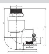
Transition elbow V2A pipe WUN V2A 90
