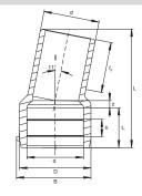
Elbow WS11 SDR 11 with spigot
